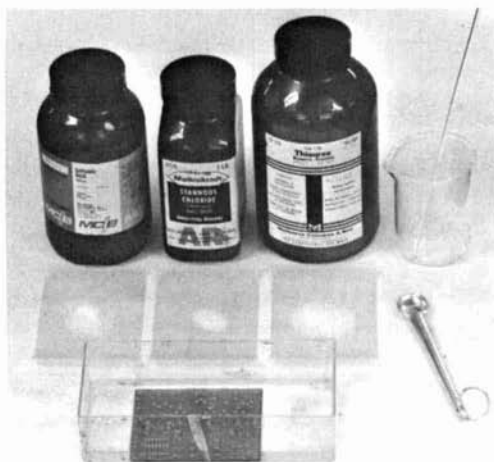
Materials for an electroless tin-plating bath.
